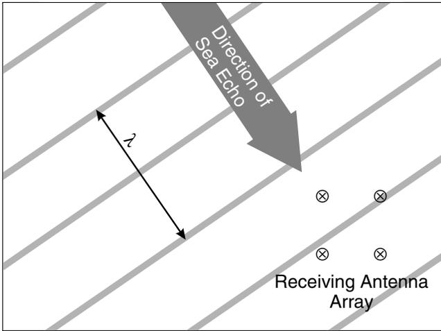
**Figure 8.** A sea echo arriving from the upper left which causes a phase difference between the antennas.
