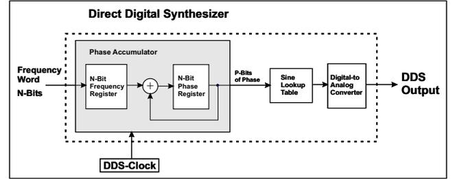
**Figure 5.** The block diagram of Direct Digital Synthesizer (DDS)
