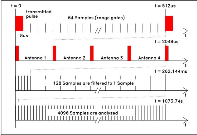
**Figure 1.** The timing used within the CODAR.
