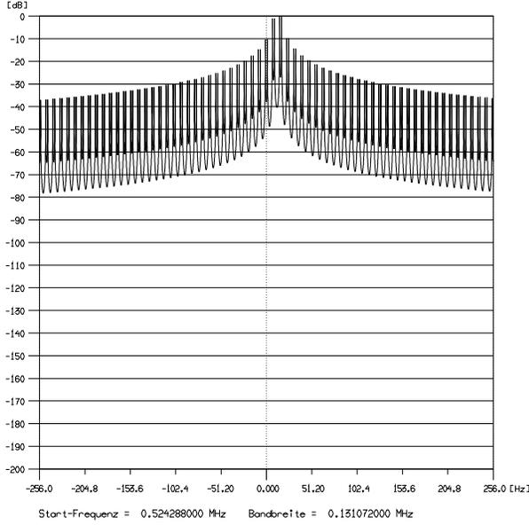
**Figure 6.** Simulation result: Sea echos at  $\pm 1.1$  Hz positioned at range cell  $1 + \frac{17}{32}$ . Due to the phase incontinuity, this signal also appears at neighbouring range cells.
