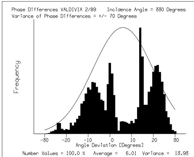
**Figure 11.** The frequency distribution of resolved incident angles using the calibrated phase difference values shown in figure 10. A simulation result showing a worst case.
