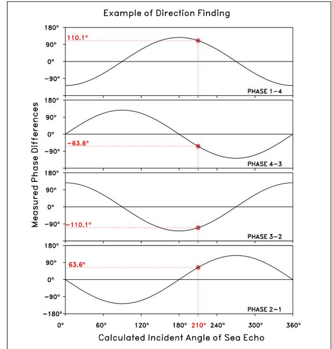
**Figure 9.** How to find the incident angle from the measured phase differences.
