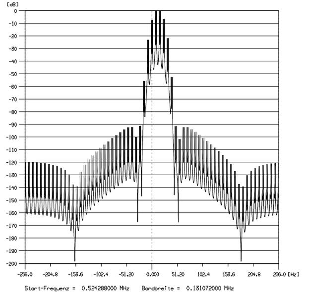
**Figure 7.** Simulation result: Sea echos at  $\pm 1.1$  Hz positioned at range cell  $1 + \frac{17}{32}$ . After applying a Blackman-Harris window, range smearing is strongly reduced.
