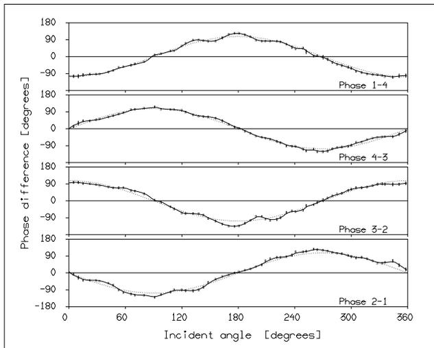
**Figure 10.** The measured phase differences for the antenna array mounted on the A-frame of RV Valdivia.
