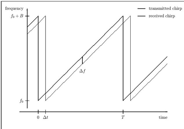
**Figure 4.** A linear frequency chirp starting at  $f_0$  with the bandwidth  $B$  and a duration  $T$ . After reaching the end frequency  $f_0 + B$ , the chirp phase contiguously starts again at  $f_0$ .
