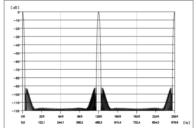
**Figure 3.** The frequency response of the digital filter used in the CODAR up to  $256 R$  with a Blackman-Harris window applied.
