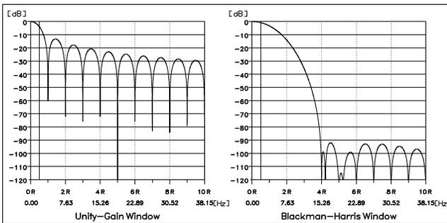
**Figure 2.** The frequency response of the digital filter used in the CODAR with a unity-gain and a Blackman-Harris window applied. All signals at frequencies higher than  $0.5 R$  are aliased back.
