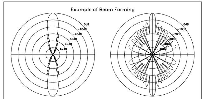
**Figure 12.** The antenna pattern of a linear array with 16 antennas at  $\lambda/2$  spacing (right side). A windowing function has to be applied to reduce side lobes (left side).
