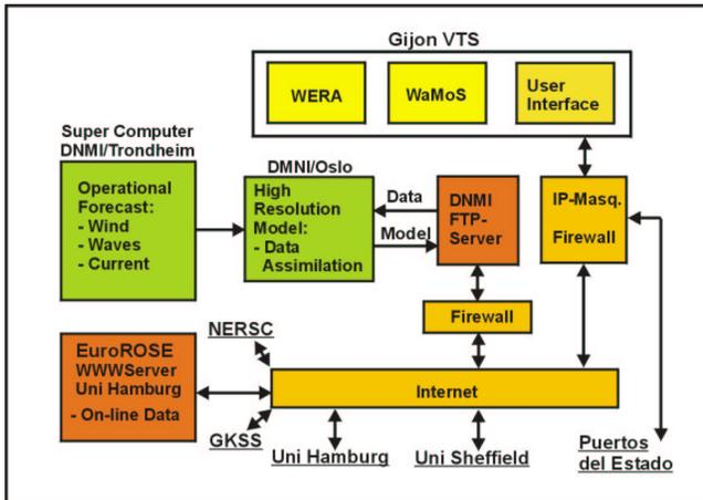
**Figure 7.** The data communication set-up used during the EuroROSE Gijon experiment. Firewalls protect sensitive system components unauthorised access.
