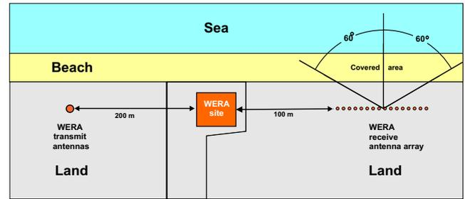
**Figure 2.** An example of a WERA HF radar installation at the coast using a linear array receive antenna. This configuration enabled simultaneous measurement of near-surface currents and ocean wave spectra.
