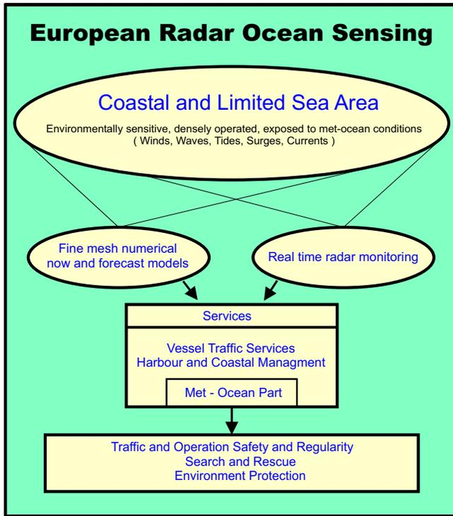
**Figure 1.** The structure of the EuroROSE system, which provides on-line now- and forecasts of currents and waves for harbour and coastal management.
