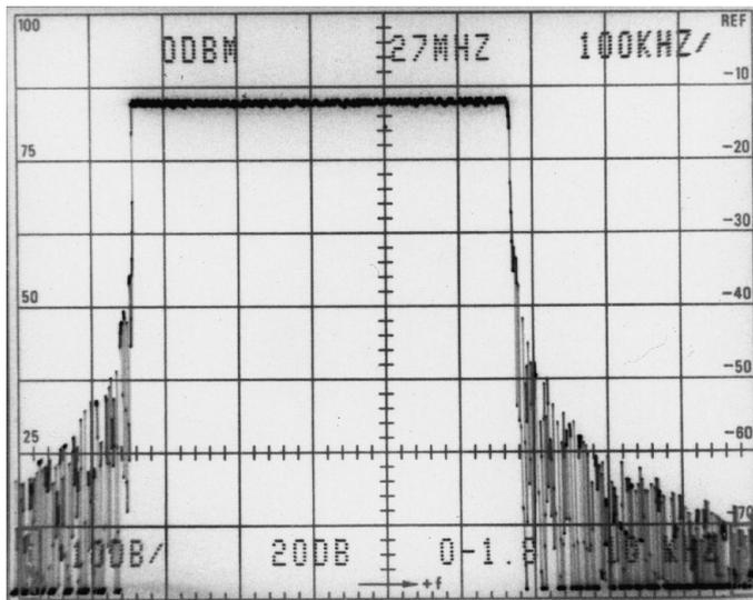
Fig. 3. The radio spectrum of a FMCW radar system at 500 kHz chirp width  $B$  and 0.26 s chirp period. The spectrum analyser's settings are 100 kHz per div. horizontally and 10 dB per div. vertically. The center frequency is about 27 MHz, the IF filter bandwidth is 10 kHz. The spectrum rapidly drops to -60 dB at 300 kHz off the radar operating frequency.
