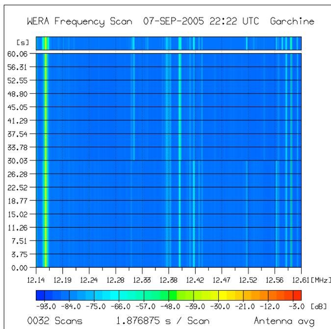
Fig. 4. A frequency scan showing the radio spectrum utilisation in the range 12.14–12.61 MHz. 32 single chirps covering the temporal variation during one minute as well as the average at the top of the figure can be seen. The colour scale represents the receiver power in dB.
