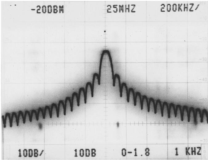
Fig. 1. The radio spectrum of a pulsed coherent radar system at  $16 \mu\text{s}$  pulse length and 2 kHz pulse repetition frequency. The spectrum analyser's settings are 200kHz per div. horizontally and 10dB per div. vertically. The center frequency is about 25 MHz, the IF filter bandwidth is 1 kHz. The spectrum covers a wide frequency frequency range and reaches -30dB at  $\pm 1$  MHz.
