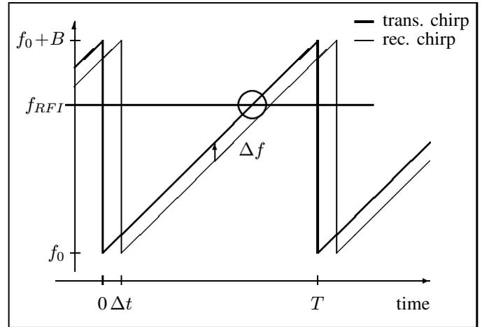
Fig. 2. Description of the FMCW radar signal: A frequency chirp starts at  $f_0$  and linearly increases the frequency with time to  $f_0 + B$  during the chirp period  $T$ . The chirp passes the operating frequency of a radio service at  $f_{RFI}$ . See text for details.
